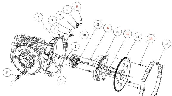
Torque converter packages available for other engines. Custom spacers, flex plates, and bell housings will be required. Please call Weddle Industries for details.
