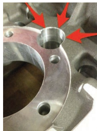
Figure 3. This area must be cleared for input coupler.
