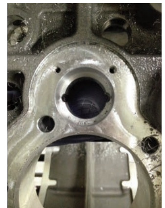
Figure 2. Modified bearing bore with notches.
