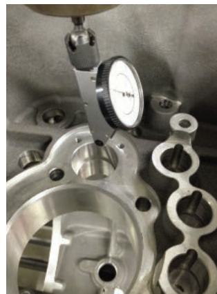
Figure 1. Indicate mainshaft bearing bore.
