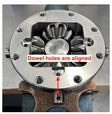
Continue tapping the long crass shaft through the opposite spider gear until the cross shaft is fully in the carrier. Check to make sure the dowel hole in the cross shaft is aligned as best as possible with the hole in carrier.
