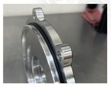
For units with (6) M8 bolts, and (2) M10 bolts around the sidecover (Arctic Cat part #2502-756): Install the o-ring around the outside register, against the outer flange of the sidecover. Do not install into the groove. Apply a light layer of moly or bearing grease on the o-ring.
