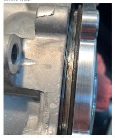
• Install the supplied output seal, using a small coating of grease on the inner lip of the seal for lubrication. It is recommended to use seal retaining compound around the outer diameter of the seal. Install seal until flush with the outer surface of the sidecover.
