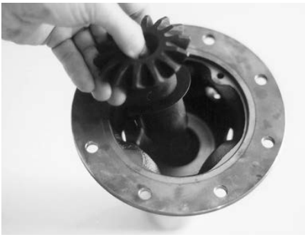
Figure 2. Place the long sidegear (with thrust washer) into the housing.
