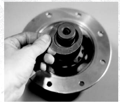
Figure 8. Place the short sidegear with thrust washer onto the top driver with the teeth meshed.
