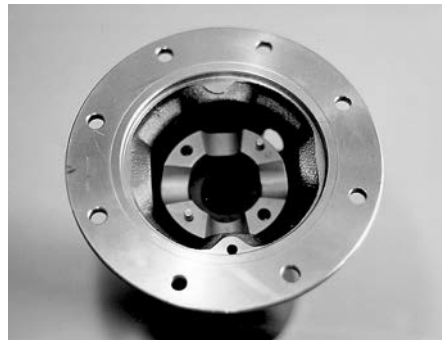
Figure 3. Place a driver onto the sidegear with teeth meshed.
