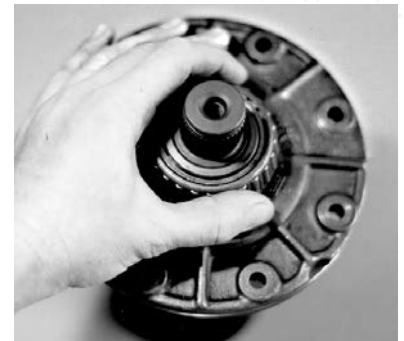
Figure 9. Place the differential cover onto the housing, making sure to line up the bolt holes.
